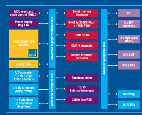
DMA: Direct memory access RTC: Real-time clock RWW: Read-while-write SSP: Synchronous serial peripheral
