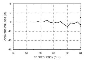
Note: Measured Performance Characteristics (T<sub>OP</sub> = 25°C)
