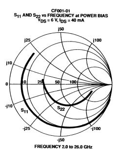
Typical Scattering Parameters, Common Source (S-Parameters Include Bonding Wire Parasitics)
