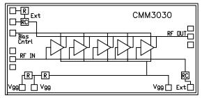
controlled to maintain correct drain current and thus drain voltage. The typical gate voltage needed to do this is 0.0V. Typically the gate is protected with Silicon diodes to limit the applied voltage. Also, make sure to sequence the applied voltage to ensure negative gate bias is available before applying the positive drain supply.
