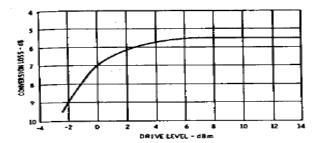
Conversion Loss vs. Drive Level: Conversion loss in an SSB system is a function of drive level (f with f and f at approximately 3 GHz and f level at -6 dBm.
