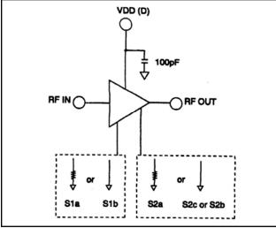
3. Nominal bias is obtained with on-chip resistors by grounding pads S1b and S2b.
