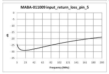
Electrical Specifications:  $Z_0 = 75\Omega$ ,  $T_A = 25^{\circ}C$ ,  $P_{in} = 0dBm$
