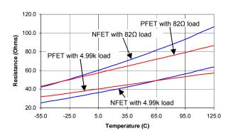
12. Output resistance were measured under the condition of  $V_{CC}$  = 5.0V,  $V_{OPT}$  = 5.0V, and  $V_{EE}$  = -5.0V, with load resistors from outputs to ground.
