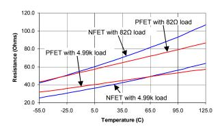
11. Output resistance were measured under the condition of  $V_{CC} = 5.0V$ ,  $V_{OPT} = 5.0V$ , and  $V_{EE} = -5.0V$ , with load resistors from outputs to ground.
