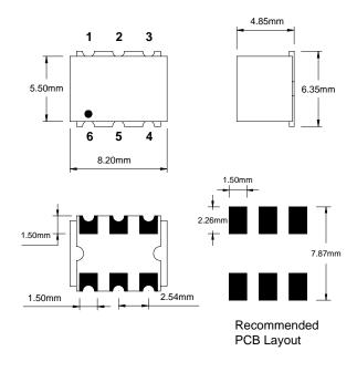
Dimensions in mm, Tolerance: .xx  $\pm$  0.3 , unless otherwise stated. Drawing not to scale.
