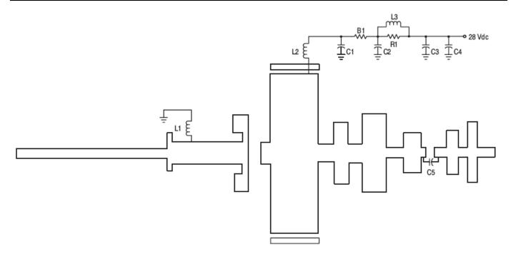
Board Material – Teflon® Glass Laminate Dielectric Thickness – 0.30",  $\epsilon_\Gamma$  = 2.55", 2.0 oz. Copper
