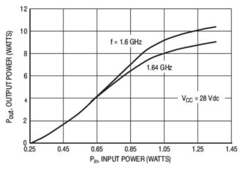
Figure 3. Output Power versus Input Power
