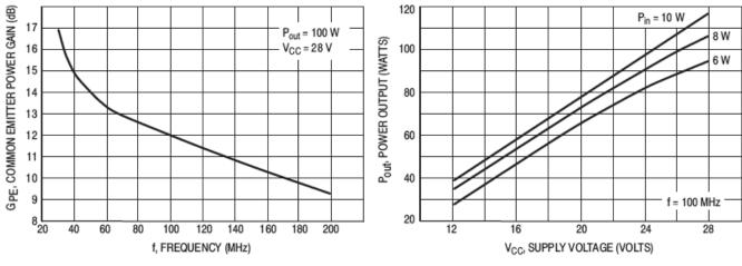
Figure 6. Power Gain versus Frequency
