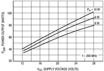
Figure 8. Power Output versus Supply Voltage
