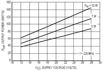
Figure 4. Output Power versus Supply Voltage
