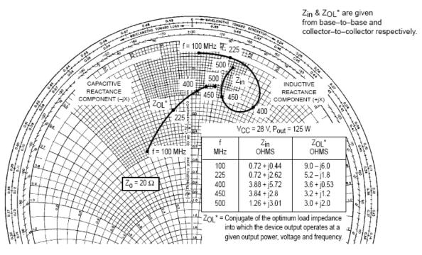
Figure 6. Series Equivalent Input/Output Impedance
