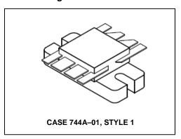
The MRF392 is two transistors in a single package with separate base and collector leads and emitters common. This arrangement provides the designer with a space saving device capable of operation in a push–pull configuration.
