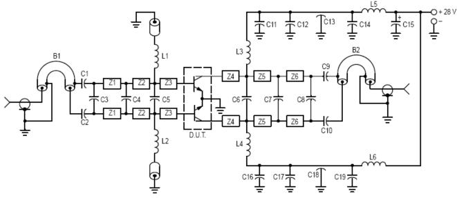
C1, C2 — 240 pF, 100 Mil Chip Cap (ATC) or Equivalent
