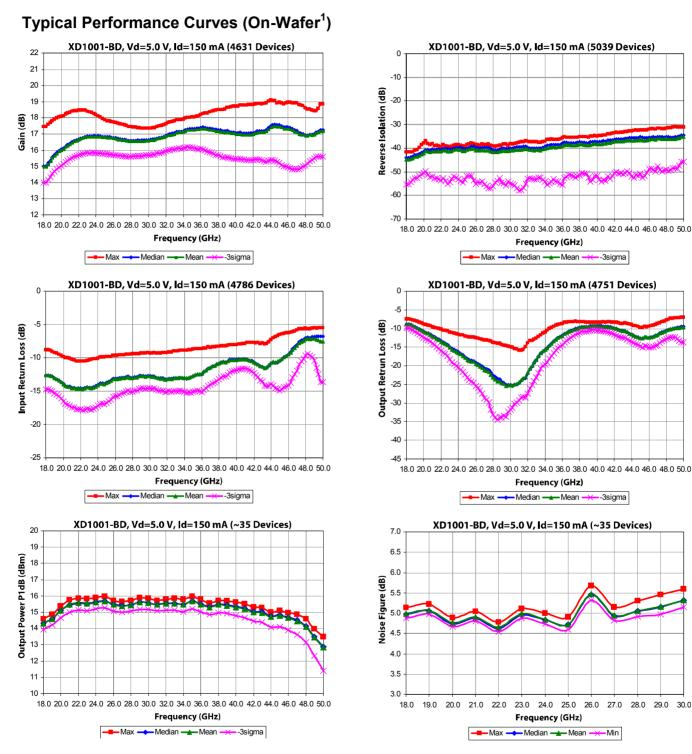
Note [1] Measurements – On-Wafer data has been taken using bias conditions as shown. Measurements are referenced 150 um in from RF In/Out pad edge. For optimum performance M/A-COM Tech T-pad transition is recommended. For additional information see the M/A-COM Tech "T-Pad Transition" application note.
