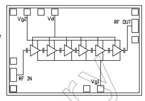
maintain correct drain current and thus drain voltage. The typical gate voltage needed to do this is 0.0V. Typically the gate is protected with Silicon diodes to limit the applied voltage. Also, make sure to sequence the applied voltage to ensure negative gate bias is available before applying the positive drain supply.
