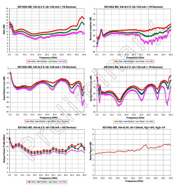
**Note [1] Measurements** – On-Wafer data has been taken using bias conditions as shown. Measurements are referenced 150 um in from RF In/Out pad edge. For optimum performance Mimix T-pad transition is recommended. For additional information see the Mimix "T-Pad Transition" application note.
