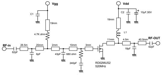
L1:Enameled wire 9 Turns,D:0.43mm,2.46mmm O.D C1,C2:1000pF,0.0022µF in parallel
