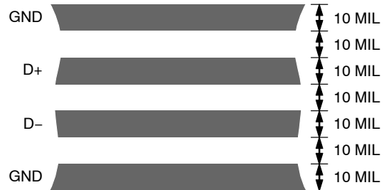
Figure 18. Arrangement of Signal Tracks
