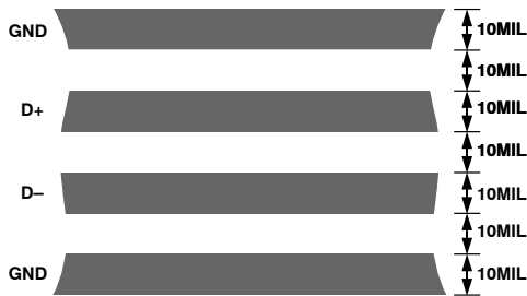
Figure 19. Arrangement of Signal Tracks
