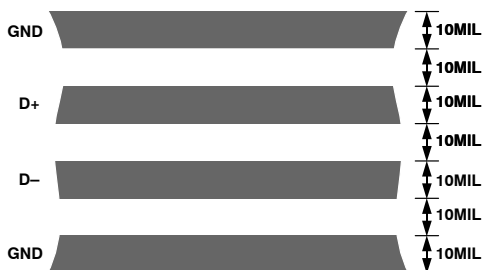
Figure 18. Arrangement of Signal Tracks
