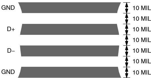
Figure 18. Typical Arrangement of Signal Tracks
