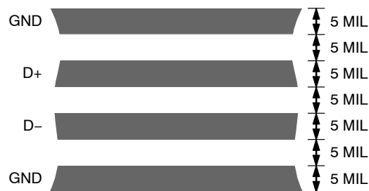
Figure 28. Arrangement of Signal Tracks
