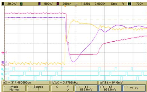
Figure 11. Typical Transient Response for Design Example Load Release 1-Vo, 3-COMP, 4-TRDET, D0~D2-PWM1~3
