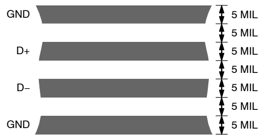
Figure 23. Typical Arrangement of Signal Tracks
