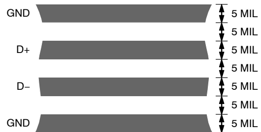
Figure 34. Typical Arrangement of Signal Tracks
