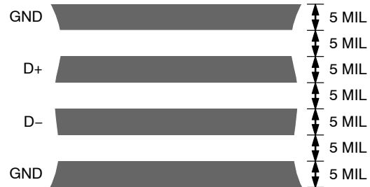
Figure 23. Typical Arrangement of Signal Tracks
