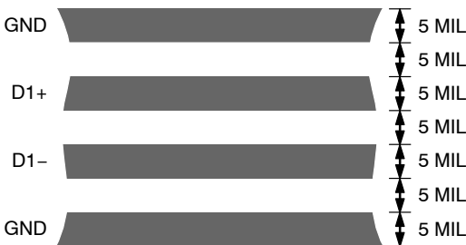
Figure 17. Arrangement of Signal Tracks
