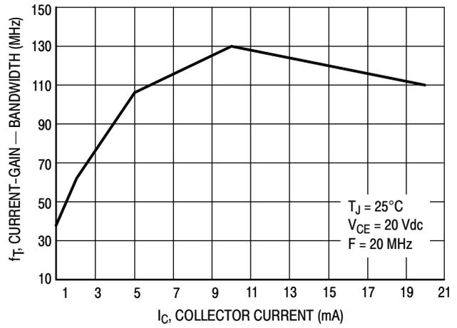
Figure 3. Current-Gain - Bandwidth
