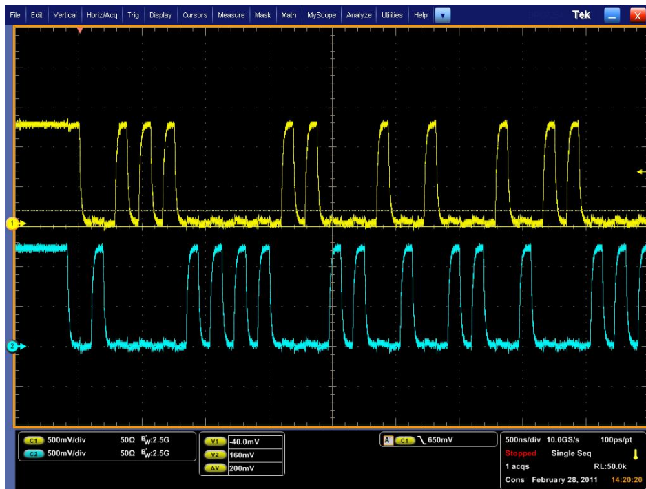
Figure 8. EMI4182 MIPI D-PHY LP Mode Measured Results
