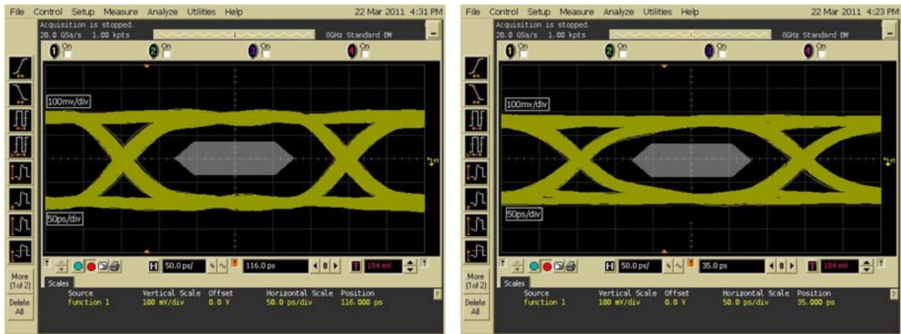
Figure 10. EMI4183MU Measured Eye Diagram @ 3.4Gbps (EVB through on left, EVB with EMI4183MU on right)
