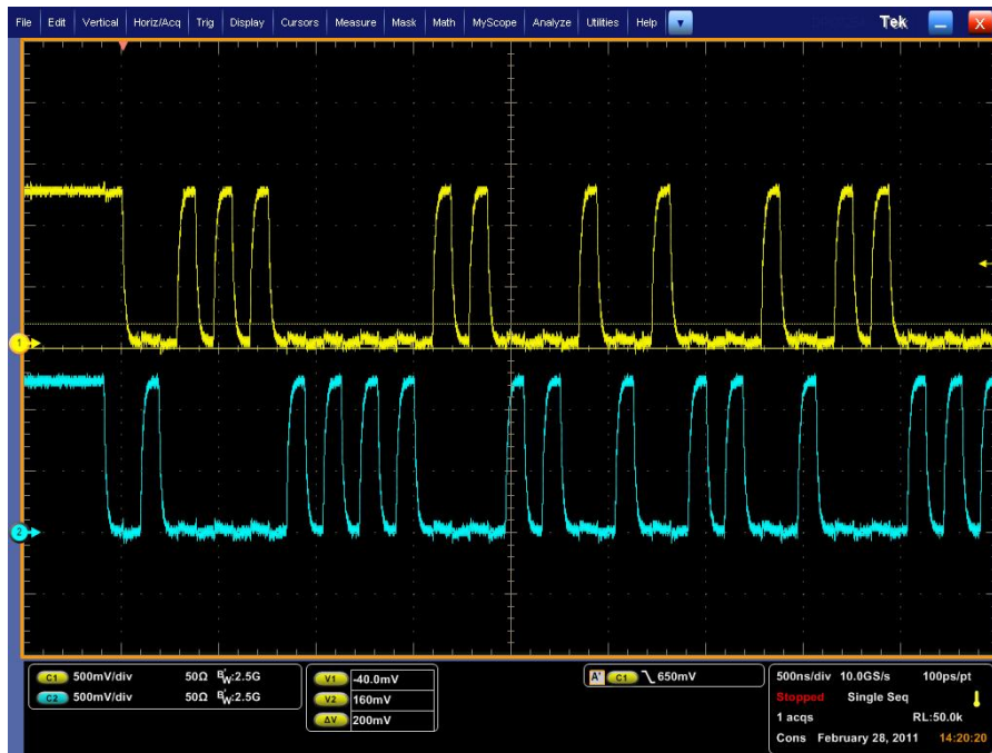
Figure 5. EMI4192 MIPI D-PHY LP Mode Measured Results
