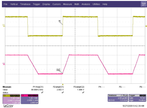
Figure 10. Non-Inverting Large Signal Step Response
