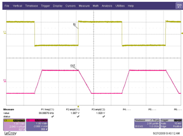
Figure 12. Inverting Large Signal Step Response
