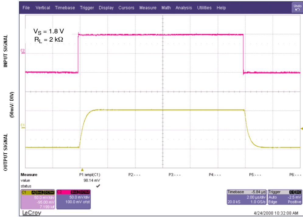
Figure 16. Small Signal Noninverting Response
