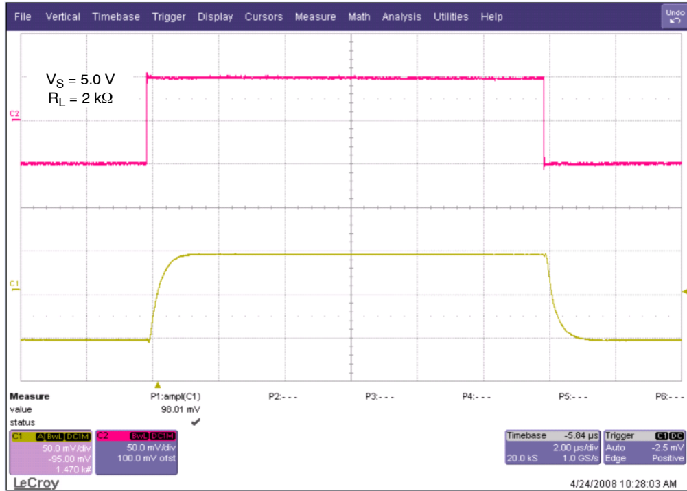
Figure 18. Small Signal Noninverting Response
