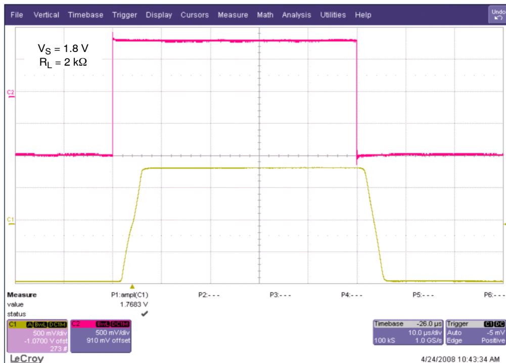
Figure 18. Small Signal Noninverting Response
