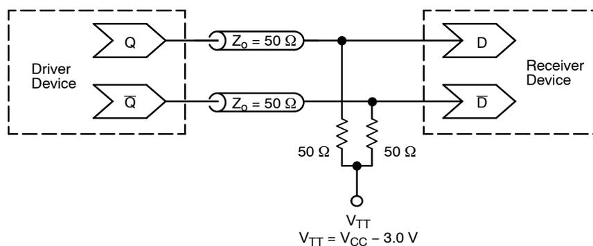
**Figure 1. Typical Termination for Output Driver and Device Evaluation**
