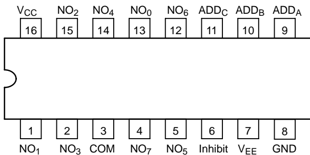
Figure 1. Pin Connection (Top View)
