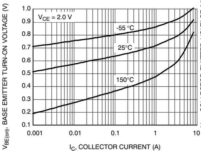
**Figure 5. Base Emitter Turn-On Voltage vs. Collector Current**
