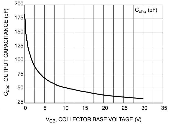
Figure 8. Output Capacitance
