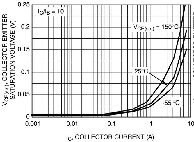
**Figure 1. Collector Emitter Saturation Voltage vs. Collector Current**
