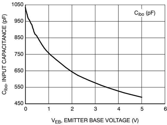
Figure 7. Input Capacitance
