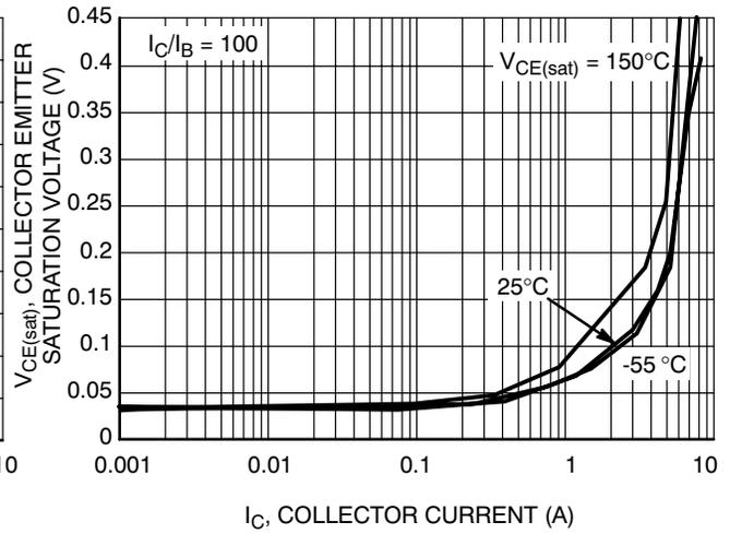
**Figure 2. Collector Emitter Saturation Voltage vs. Collector Current**
