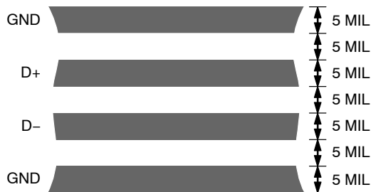
Figure 22. Typical Arrangement of Signal Tracks
