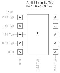
Figure 1. PCB Metal Land Pattern (Top View)
