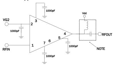
NOTE: Drain Bias (Vdd) must be applied through a broadband bias tee or external bias network.
