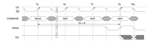
Burst Length = 4 in the cases shown Shown with nominal  $t_{AC}$  and nominal  $t_{DSDQ}$
