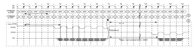
Note: 1.tRRD2 is Row Active to Row Active Delay between two independent 8banks.(2CS mode)
