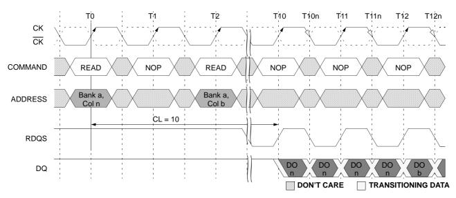
Note: 1. DO n (or x or b or g) = data-out from column n (or column x or column b or column g).
