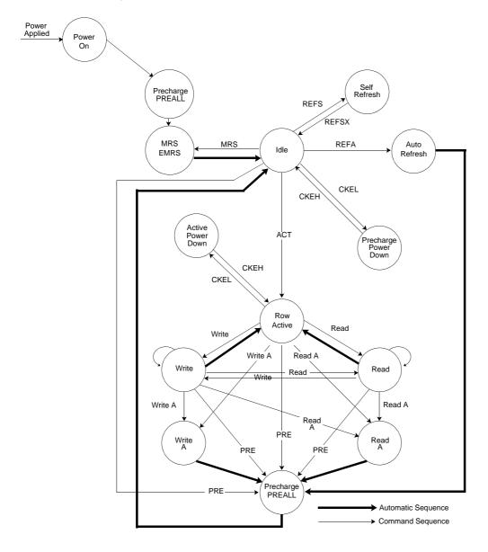
PREALL = Precharge All Banks MRS = Mode Register Set EMRS = Extended Mode Register Set REFS = Enter Self Refresh REFSX = Exit Self Refresh REFA = Auto Refresh CKEL = Enter Power Down CKEH = Exit Power Down ACT = Active Write A = Write with Autoprecharge Read A = Read with Autoprecharge PRE = Precharge
