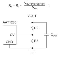
Figure 2: Over-Voltage Protection Circuit.
