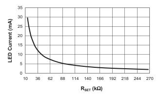
Figure 1: LED Current vs. R<sub>SET</sub> Values.
