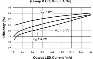
Efficiency vs. LED Current (Group A and B On)
