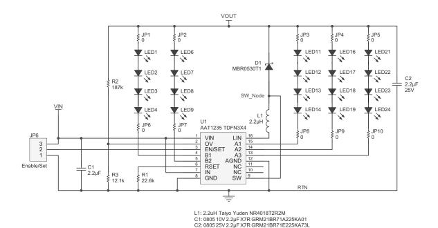
Figure 3: A AAT1235-based High Efficiency White LED Driver Schematic.
