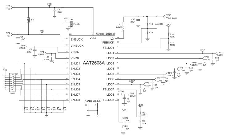
Figure 1: AAT2608A Evaluation Board Schematic.
