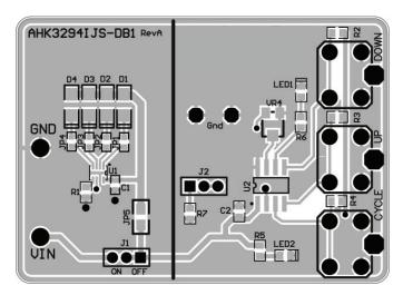
Figure 5: AHK3294 Evaluation Board Top Side Layout.
