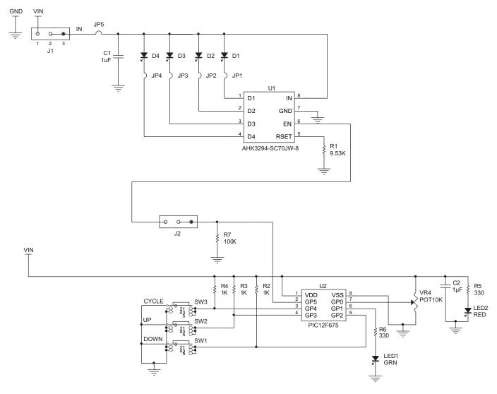
Figure 4: AHK3294 Evaluation Board Schematic.
