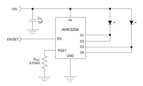
Figure 3: Higher Current Dual LED Application.
