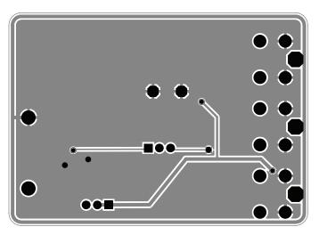
Figure 6: AHK3294 Evaluation Board Bottom Side Layout.
