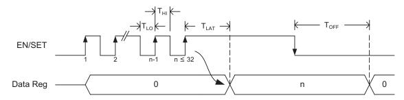
Figure 1: S<sup>2</sup>Cwire Serial Interface Timing.
