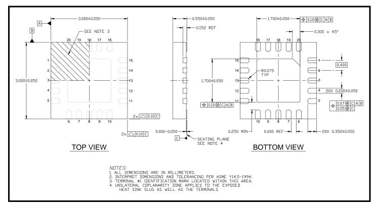
Figure 5: SE2611T Package Diagram
