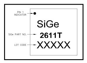
Figure 4: SE2611T Branding and Pin 1 Location
