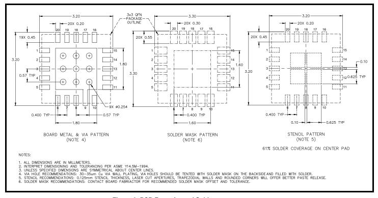
Figure 6: PCB Footprint and Solder pattern
