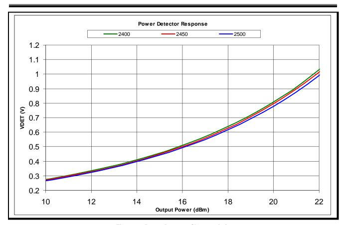
Figure 3: Power Detector Characteristic
