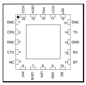
Figure 2: SE2611T Pin out (Top View through Package)
