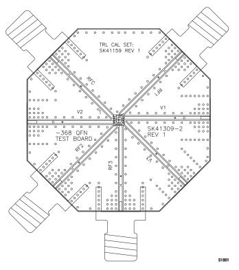
Figure 13. SKY13346-368LF Evaluation Board Assembly Diagram
