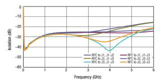
Figure 8. Port to Port Isolation vs Frequency (Insertion Loss Ports to Off Ports)
