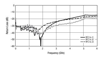
Figure 9. Input Return Loss vs Frequency
