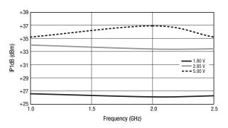
Figure 10. Input 1dB Compression Point vs Frequency
