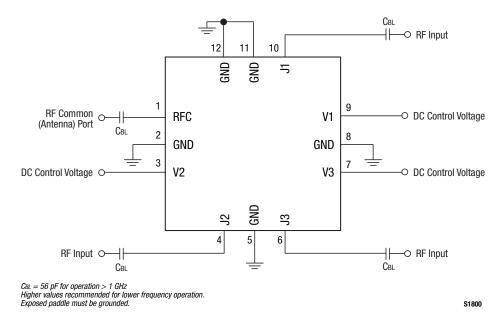
Figure 12. SKY13346-368LF Evaluation Board Schematic
