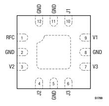
Figure 2. SKY13346-368LF Pinout – 12-Pin QFN (Top View)
