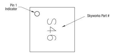
Figure 15. Typical Case Markings (Top View)
