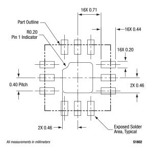
Figure 14. SKY13346-368LF PCB Layout Footprint (Top View)
