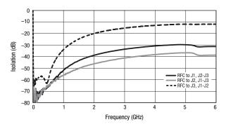
Figure 7. Port to Port Isolation vs Frequency (Off Ports to Off Ports)
