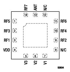
Figure 2. SKY13417-485LF Pinout – 14-Pin QFN (Top View)
