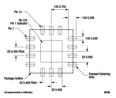
Figure 5. SKY13417-485LF PCB Layout Footprint (Top View)
