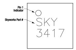
Figure 6. Typical Part Markings (Top View)
