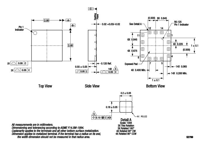
Figure 7. SKY13417-485LF 14-Pin QFN Package Dimensions
