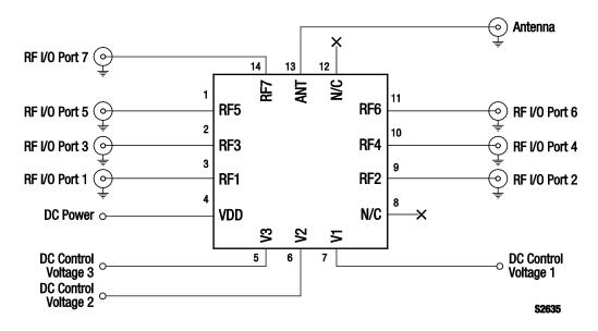
Figure 3. SKY13417-485LF Evaluation Board Schematic
