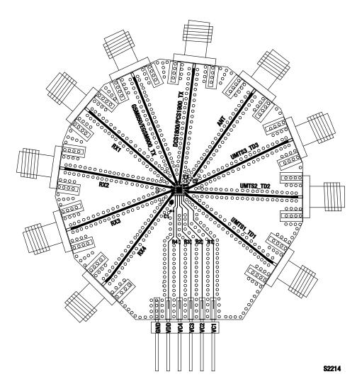
Figure 4. SKY18120-11 Evaluation Board Assembly Diagram
