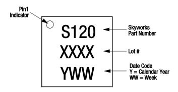
Figure 6. Typical Part Markings (Top View)
