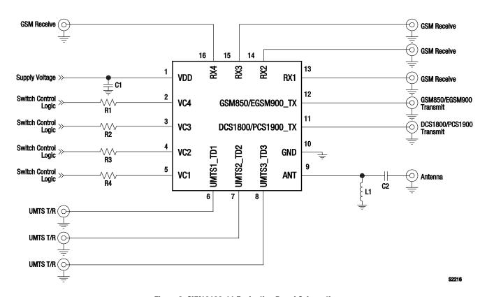
Figure 3. SKY18120-11 Evaluation Board Schematic
