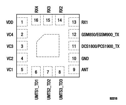
Figure 2. SKY18120-11 Pinout – 16-Pin MCM (Top View)
