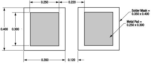
All measurements in millimeters
