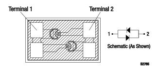
Figure 1. SMS7621-092 Pinout (Bottom View)
