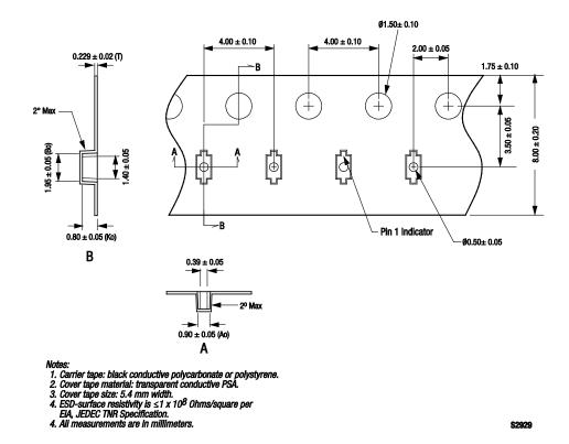
Figure 7. SC-79 Tape and Reel Dimensions
