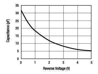
Figure 1. Capacitance vs Reverse Voltage
