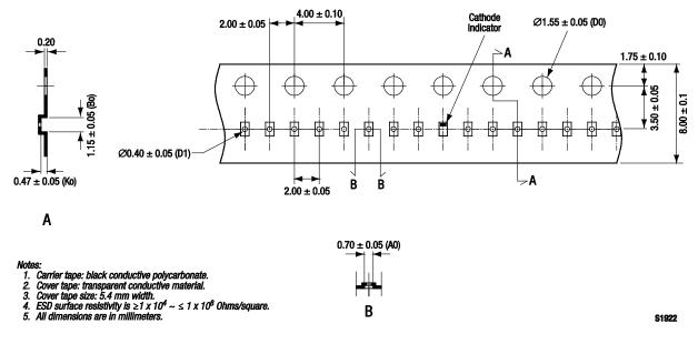
Figure 11. SOD-882 Tape and Reel Dimensions
