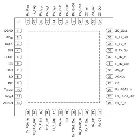
Exposed thermal pad is connected to ground.
