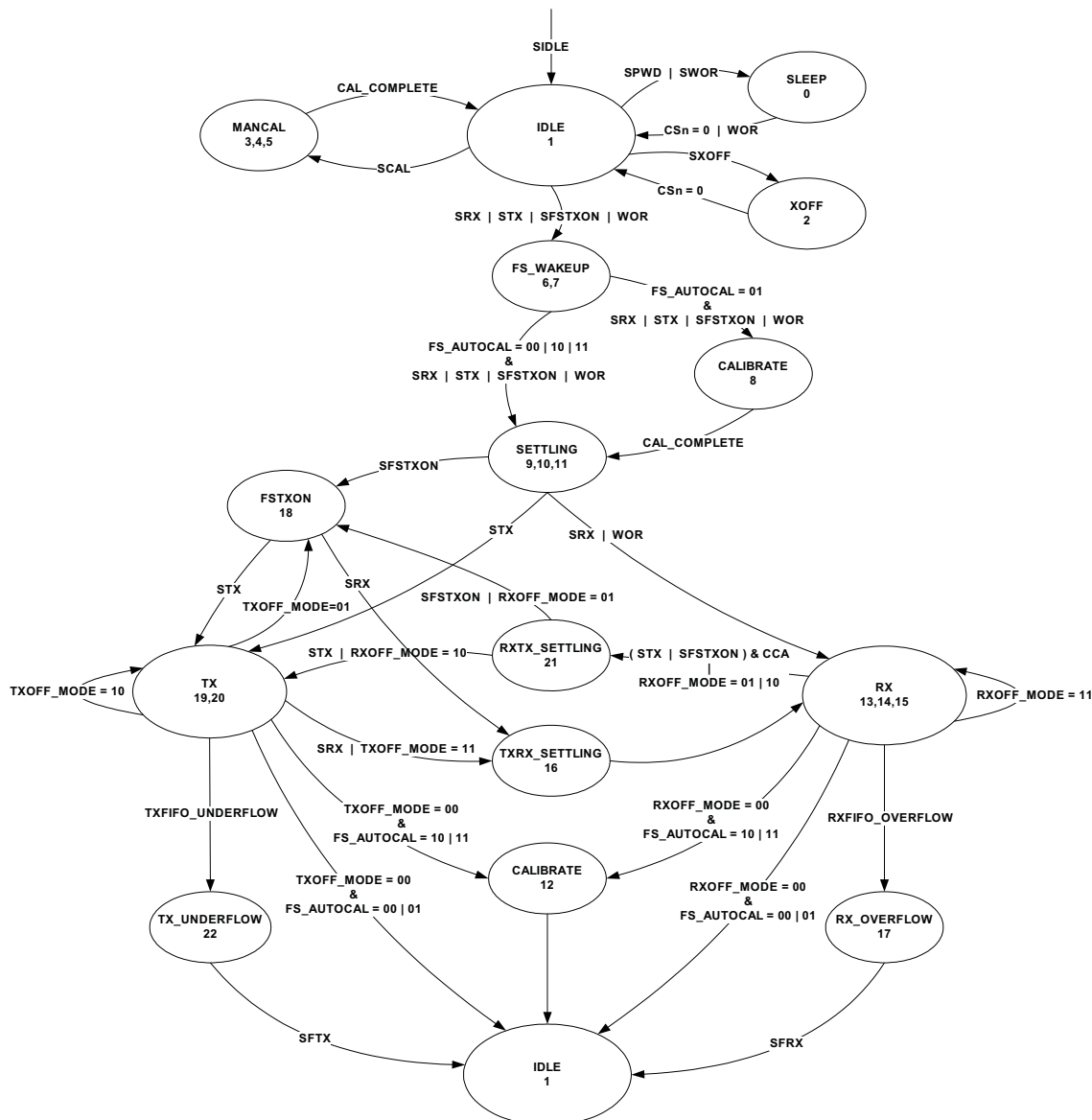
Figure 3-15. Complete Radio-Control State Diagram
